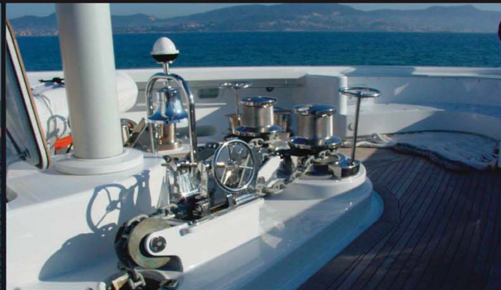
complete stainless steel anchoring system including mooring capstans and stern anchorwinch
