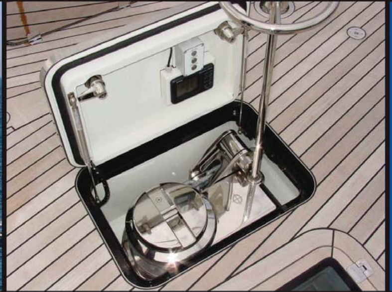
complete set of two Type 3 stainless steel anchor winches
