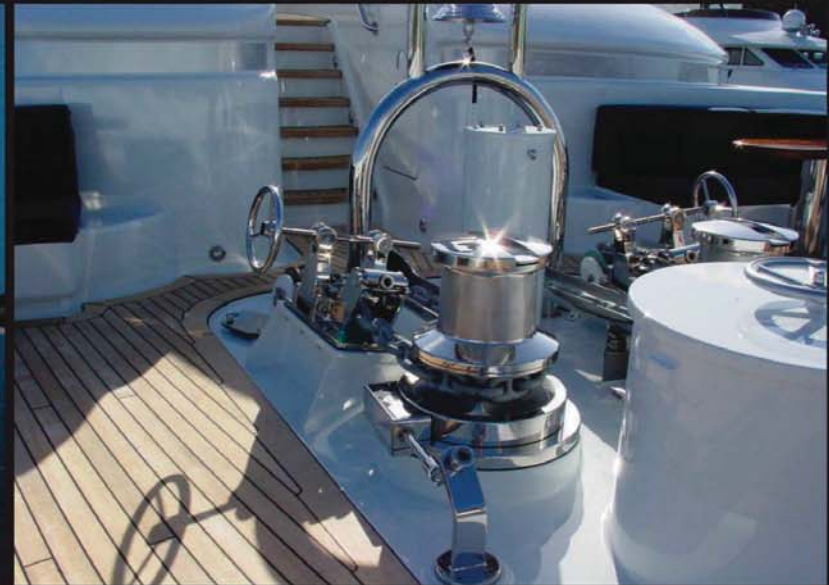
complete stainless steel anchoring and mooring system
