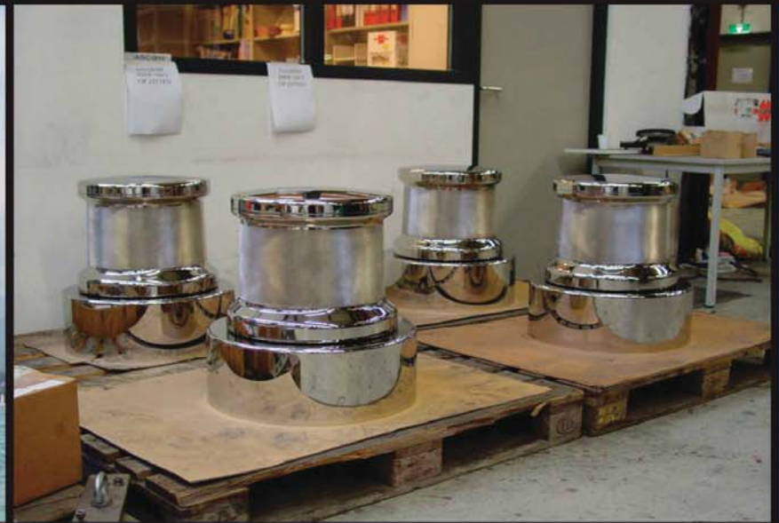
6 stainless steel custom designed mooring capstans
