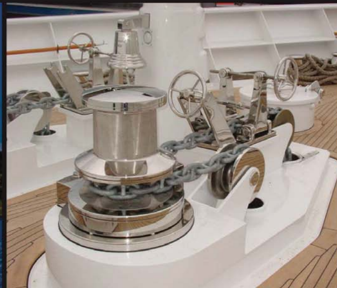
complete stainless steel anchoring and mooring system including rollers and stoppers for 28mm studlink chain
